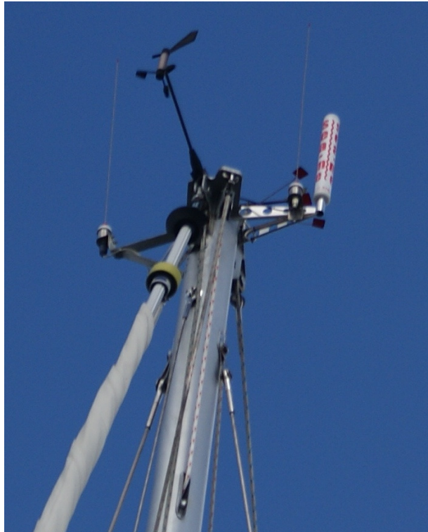
Masthead with inner forestay on tang about 300mm below With AIS, VHF, Sea Me transponder
