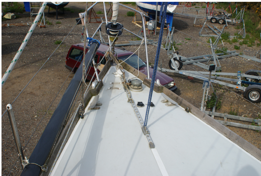
Sail track inadequate for load Blue rope downhaul will be replaced by single new stay down to Highfield lever on deck eyebolt Teak toerail being cleaned and varnished this summer
